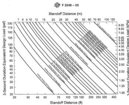
ASTM F 2248 graphical relationship between standoff distance, TNT charge mass, and 3-second equivalent design load.
