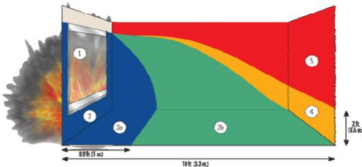
The various glass performance conditions established by GSA and ISC. Conditions vary with respect to the travel distance of the breakage debris. Graphic Courtesy Graham Architectural Products
