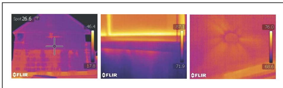
(L to R) -- Infrared thermography shows (1) moisture infiltration from the window, penetration and horizontal sealant joint behind EIFS cladding; (2) air infiltration at an existing windowsill; and (3) air infiltration at a sprinkler pipe penetration.
